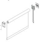
Below Ceiling (With fascia) Dimensions Small Large c A 98mm 117mm B 30mm 41mm C 84mm 115mm
