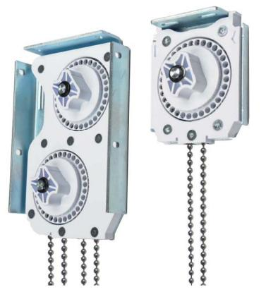
Located within the fixing bracket, rather than on the end of the tube, the ball bearing clutch is designed for the most demanding applications and provides smooth, quiet operation even for large blinds. The control chain hangs directly below the bracket, further improving stability.
