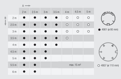
(A: Width / B: Height) The maximum surface always depends on available fabric widths and fabric weight. Any system 4m or above in width will be supplied with the profile 4957 (110 mm tube).
