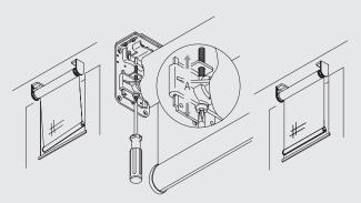
Vertical adjustment of the system (A) allows the head tube to be levelled.
