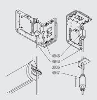
4946 Top fastener 4948 Wire rope (1.5mm) 3036 Bracket 4947 Bottom fastener
