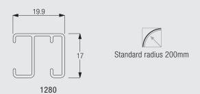
The standard radius is recommended for optimal operation. The minimum possible radius is 150mm.
